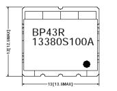
TOLERANCE UNLESS OTHERWISE SPECIFIFD : ±0.3 UNIT: mm ● INPUT PORT
