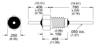
12-28 UNF-2A THREAD (X.XX) = MILLIMETERS
