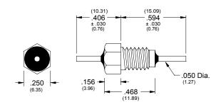
12-28 UNF-2A THREAD (X.XX) = MILLIMETERS
