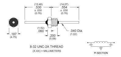
Capacitance: 1000 pF Min. Dissipation Factor: 5% Max. Working Volts DC: 100\*
