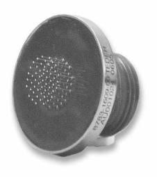
A filtered connector for ground mobile military applications based on D38999/24 Jam Nut connector with a custom low profile back shell (less than the standard connector depth). It contains 28V/12A power line filter, double L section filter with Fco=6kHz and a diversity of additional signal filters.
