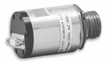
A220V/5A/50-60Hz/1 phase power line filter for telecom and military applications, DM filters and CM filters. The filter has Fco= 1kHz combined with lightening transient protection (20 J Pulse energy). The filters are integrated in a D38999/24 Jam Nut connector with a special extended back shell.
