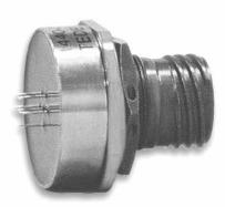
A filtered connector and an EMP protection for military applications with special back shell design. A 28V/10A Per MIL-STD-1275 power line filter and an EMP protection built in a low profile connector with the same depth as the standard one.
