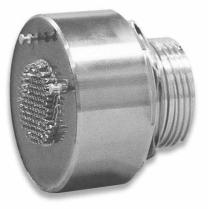
A filter connector for military applications, based on D38999/24 Jam Nut connector with the custom back shell. A power line filter and signal line filter are enclosed in its housing with a high filter attenuation from 1kHz up to 1GHz.
