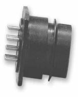
A custom-design connector developed by Corry Micronics, Inc. with an EMI filter for use in military applications. It features easy and quick mating and disconnecting and contains PI filters for frequencies ranging from 10kHz to 1GHz.
