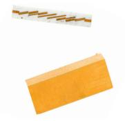
The next two 5G bands for the United States market are 27.5-28.35GHz and 37-40GHz. At these higher frequencies Quantic Corry designs filters with either waveguide, microstrip, stripline, stabline or suspended strip line. At Quantic Corry we developed a surface mount 28GHz suspended strip line filter tailored to the RF properties of the customers circuit board assembly. The customer's application was wideband communications to a drone so weight was an important factor in design.
