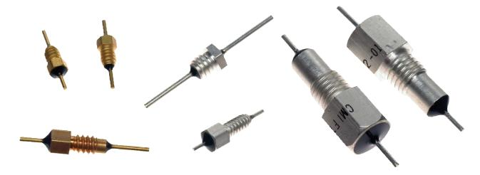
Feedthrough filters have a wire that goes all the way through the part. More current demands a larger wire, and the whole component must get bigger to surround it. Hence, filter cases get bigger, require more material, and take more machining, driving up their cost as current increases. Digital circuits generally draw less power, so you can stick with smaller filter units. For this reason, power is less of a cost driver on the digital side than on the analog side.
